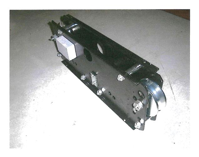
A three sheaves dynamometer is a hoist line load sensor.
